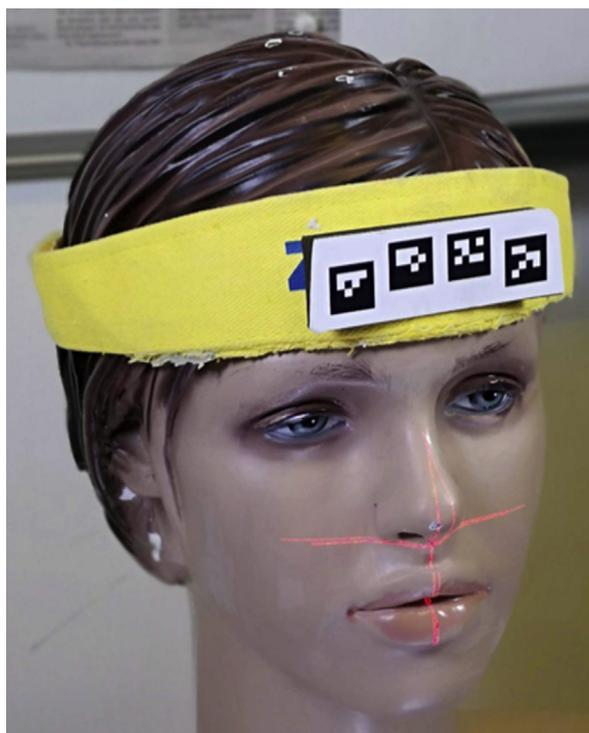
**Fig 3.** Mannequin head showing the 2 eye-safe positioning lasers projecting 1 cross each on the patient's face. The optimal working distance is obtained when both crosses coincide on the patients' midline, just below the nose.
