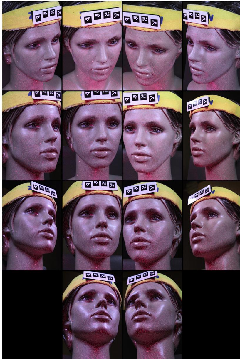
**Fig 4.** Example of the 14 camera views, as acquired from the mannequin head. The red dots are generated by the random pattern lasers, which provide additional texture to the relatively feature-sparse human facial surface.
